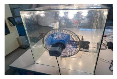
Figure (1): Model of samples is exposed to the plastic shrinkage
