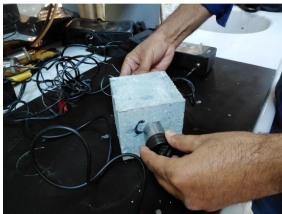
Figure (2) Ultrasonic Pulse Velocity direct test
